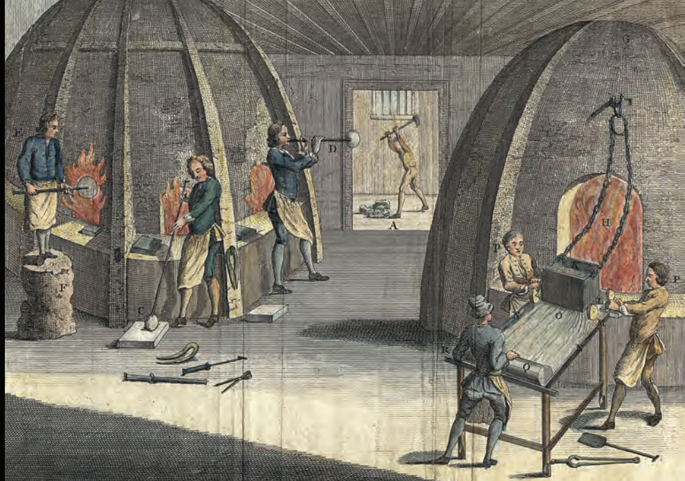
Left: The Morgan Cup. Roman Empire, first half of the first century AD Opaque white over translucent deep blue glass; blown and cased; carved, ground and polished. Right: A hand-colored engraving, which appeared in The Universal Magazine (London, 1760), depicts the manufacture of crown glass by blowing (left) and plate glass by casting (right). Glass workers were susceptible to cataract caused by the glare of the furnace.
