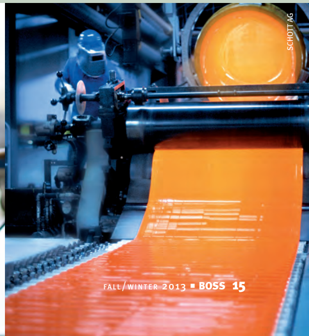
From left to right: A vase is shaped through glass blowing; raw material that has been melted in the pot at Schott in Mainz, Germany, is rolled to flat glass.
