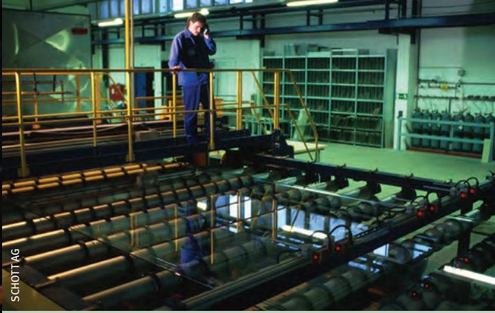
Schott Glass manufactures the world's first borosilicate glass, Borofloat, using a microfloat process.
