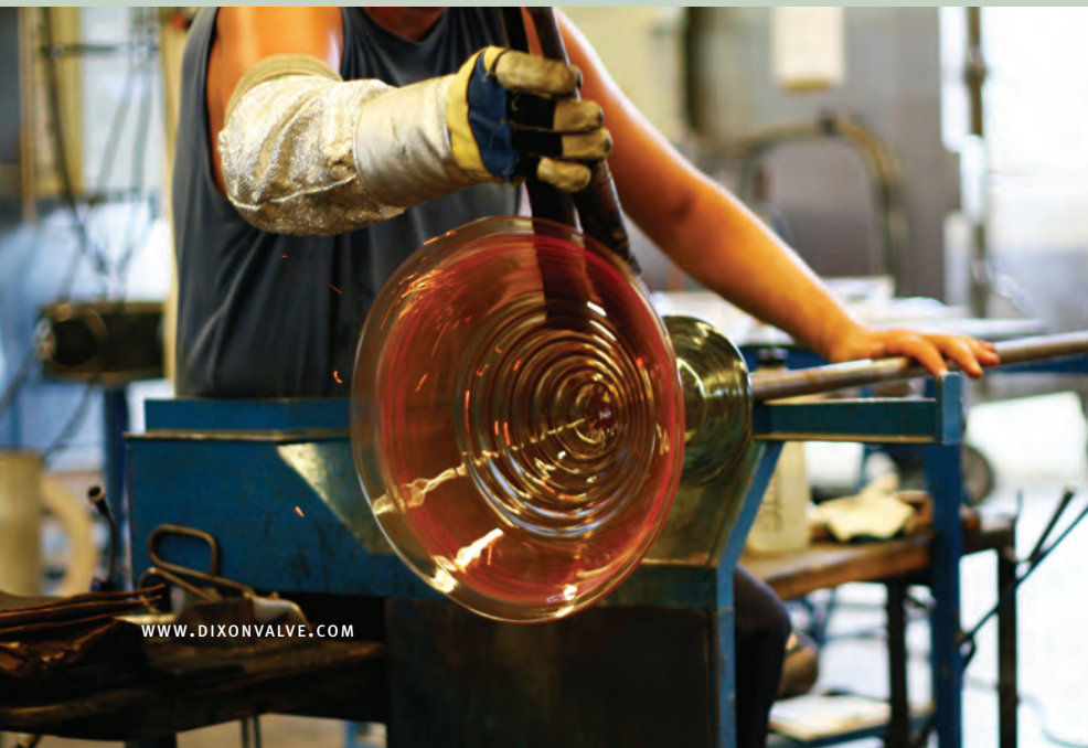
From left to right: A vase is shaped through glass blowing; raw material that has been melted in the pot at Schott in Mainz, Germany, is rolled to flat glass.
